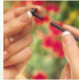
Insert diffuser bug cap into 1/4" tubing
